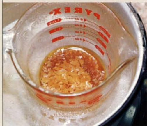
Use a shopmade double boiler to melt the wax. Most waxes will dissolve in turpentine, but it's faster to melt them (waxes used in polish melt between 145°F and 185°F). Place the wax in a heat-proof glass container, and put the container in a pot of hot water.
