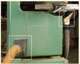
**Collect dust at two points.** Many bandsaws have dust collection below the cutting area, but Fortune also recommends installing a vacuum port at the bottom left of the lower wheel. If dust and pitch build up on the tires, the blade will not track properly. Install a brush (right) to remove dust from the lower wheel.
