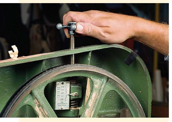
Use less than the recommended tension. For a 1/2-in.-wide blade, turn the tension gauge (above) to the setting for a %-in.wide blade. The first step in overhauling a bandsaw is to check the tires for grooves (right). If necessary, replace them.
