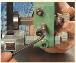
Other important guide settings. The guide assembly should be adjusted so that the metal blocks remain just behind the blade's gullets. Then the thrust bearing is set 1/32 in. behind the blade, as shown, so it contacts the blade only during use.
