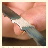
The blade weld must be smooth. A good sawblade company will weld blades precisely and grind the welded area flat. After setting the guides, turn the wheel by hand to be sure the weld passes through the guides smoothly.
