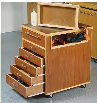
Shallow drawers hold hand tools. An open area below the top of the cabinet keeps tools within reach but out of the way. The cabinet's top has enough overhang for attaching clamps.
