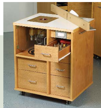
Router table holds parts and accessories. This rolling router table is equipped with a router lift. The lift is offset to accommodate drawers, bits, and accessories. Dust-collection ports are built into the fence and cabinet back.
