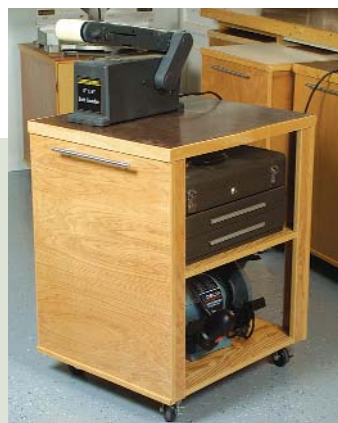
There's no such thing as too much storage. Two tall, open shelves are used for storing large objects such as a toolbox, benchtop grinder, and belt sander.
